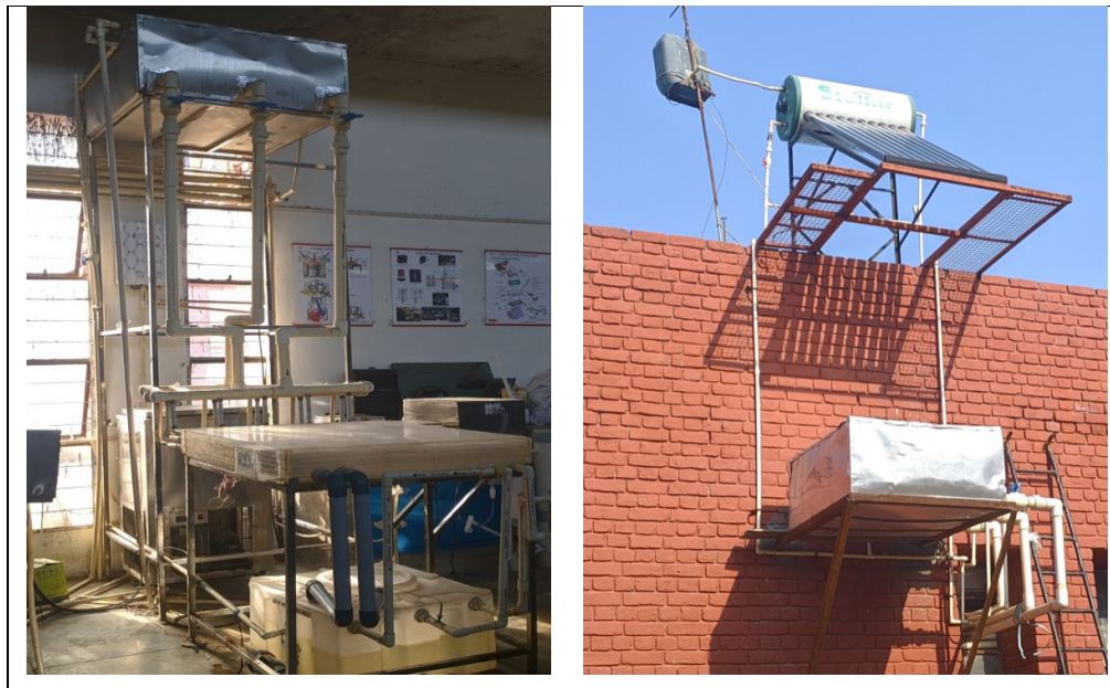
Fig. 4. Experimental setup for the dehumidification system.
